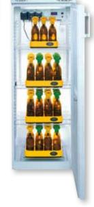
the OxiTop® Control system. Data can be recalled through the closed glass door, to avoid temperature fluctuations caused by opening the door.
